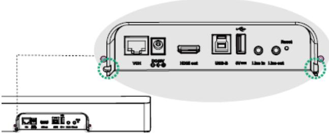
2 Fit part A of the cable cover into the slots.
